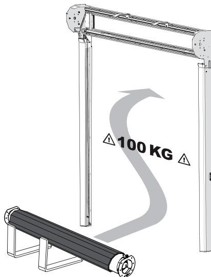
Install the top roller together with the door panel.
