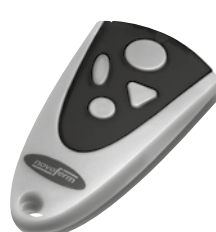
Mini-Novotron 504 hand transmitter 4-channel, 433 MHz, KeeLoq rolling code
