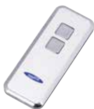
Mini-Novotron 522 Design hand transmitter 2-channel, 433 MHz, KeeLoq rolling code
