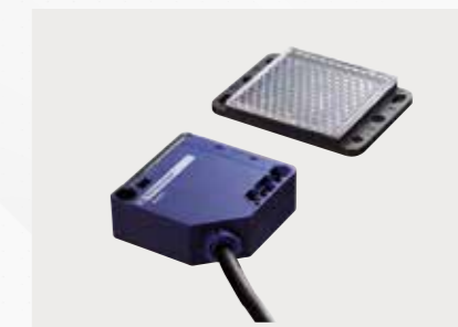
Extra 628 reflection light opto sensor 24-240 V AC, 12-240 V DC, IP 54 Range: 5 m Can only be used as a pulse generator
