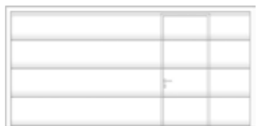
Asymmetrical arrangement for garage door widths above 3500mm - optionally on the right with right hand hinge.
