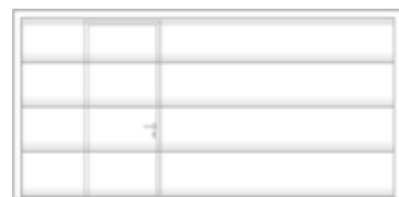
Asymmetrical arrangement for garage door widths above 3500mm - optionally on the left with left hand hinge.
