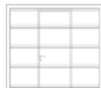
Symmetrical arrangement for garage door widths up to 3500mm.
