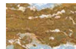
Galvanised Steel 20 µm after 6 weeks
